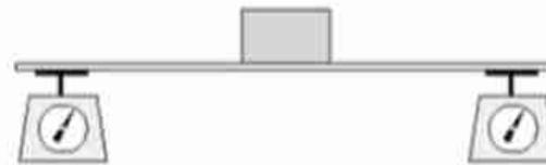
With the object in the middle, the scales show the same reading: Half the weight of the object
