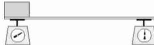
With the object on the left, one scale reads twice the original reading, and the other goes to zero
