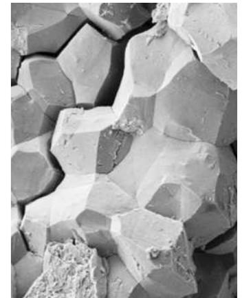
▲ The scanning electron micrograph shows intergranular failure due to hydrogen-induced cracking.
