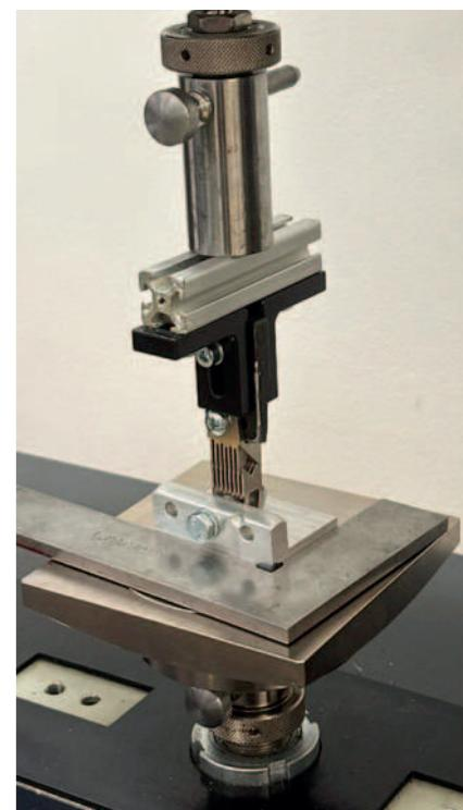
▲ Crimping using a test bench to determine the crimping force
