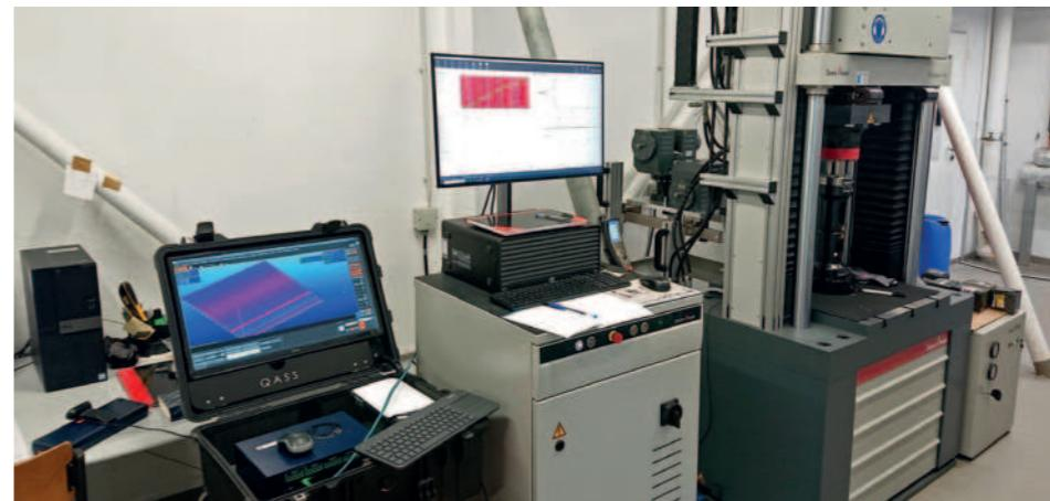
◀ Use of Prof Ralf Glienke's measurement technology in a laboratory test setup: Innovative monitoring of cyclically loaded screws.
