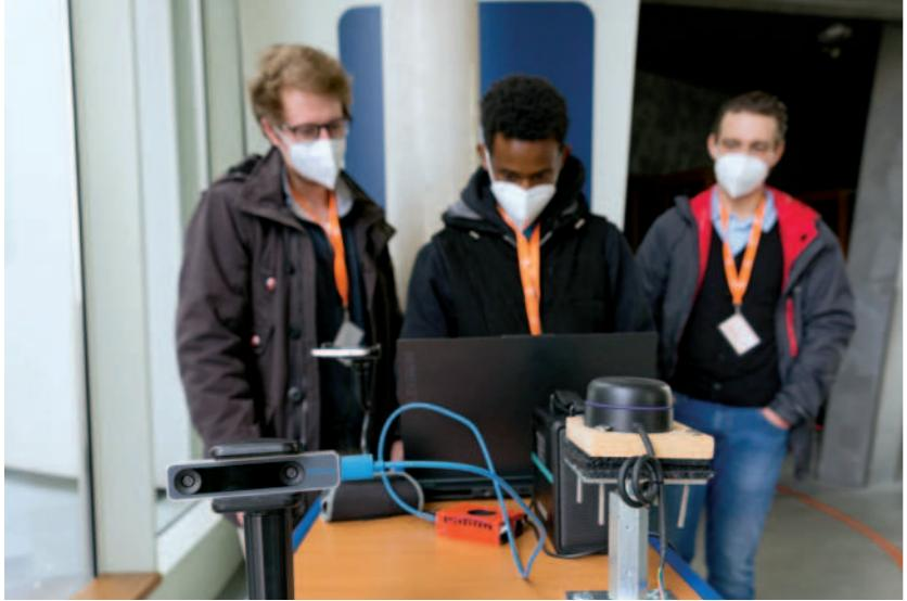
▲ Test run at the OZEANEUM Stralsund, Measuring the room using a LIDAR and a 3D camera
