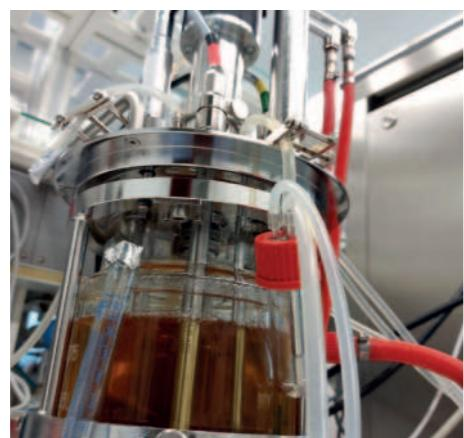
► Laboratory bioreactor for the production of cannabinoid precursors with *Dictyostelium*
